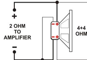
**2 X DUAL VC 2 OHM SPEAKERS WITH SERIES VOICE COILS, ALL IN PARALLEL**
