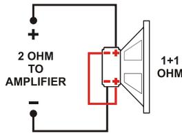
Please note that the minimum impedance load for single Cadence Q Series amplifiers is 2 ohm stereo and 4 ohm mono bridged.
