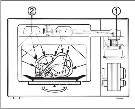
In a microwave oven there is a high-frequency tube called a magnetron ①. This converts electrical energy into microwaves. These microwaves are distributed evenly throughout the oven interior by a metal fan blade known as a stirrer ②, rebounding off the metal sides of the oven interior and thereby reaching the food from all sides. Microwave distribution is improved by engaging the turntable.
