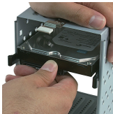
5.5 Insert the railed 3.5" HDD into the 3.5" HDD drive bay
