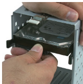
No screw needed for 3.5" HDD
