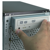
3.4 Insert the railed 5.25" device into the 5.25" drive bay
