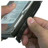
5.4 Attach rails to both sides of the 3.5" HDD.
