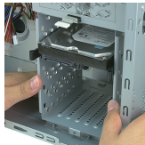
5.6 Slide the HDD cage back and fasten the thumb screws.
