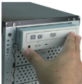
No screw needed for 5.25" device
