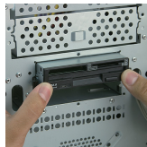
4.4 Insert the railed 3.5" device into the 3.5" drive bay.
