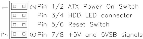
**ATX Power ON Switch: Pins 1 and 2**
