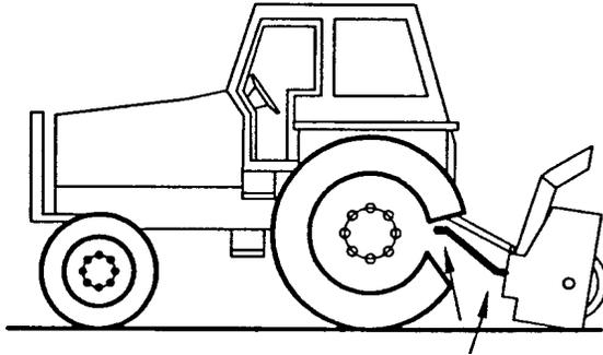
**Unequal Angles at Driveline Joints**
