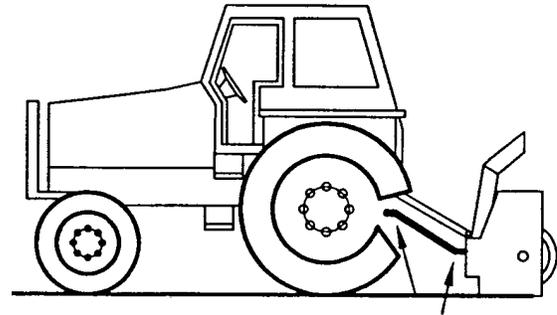
**Equal Angles at Driveline Joints**
