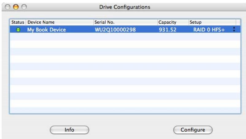
1. To configure or change the RAID setting, click on a device from the menu to display the popup menu. The checkmark indicates the current RAID configuration.
