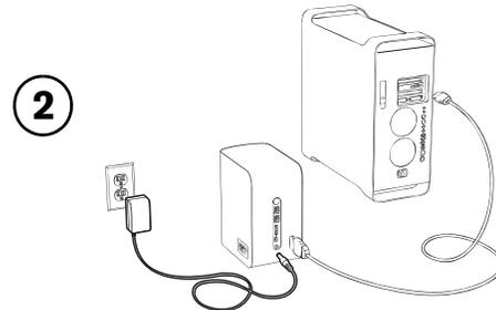
7. Connect the adapter's DC cable plug to the DC power input at the rear panel of the product. Verify that plug type of your wall power adapter is the correct plug type for your region.
