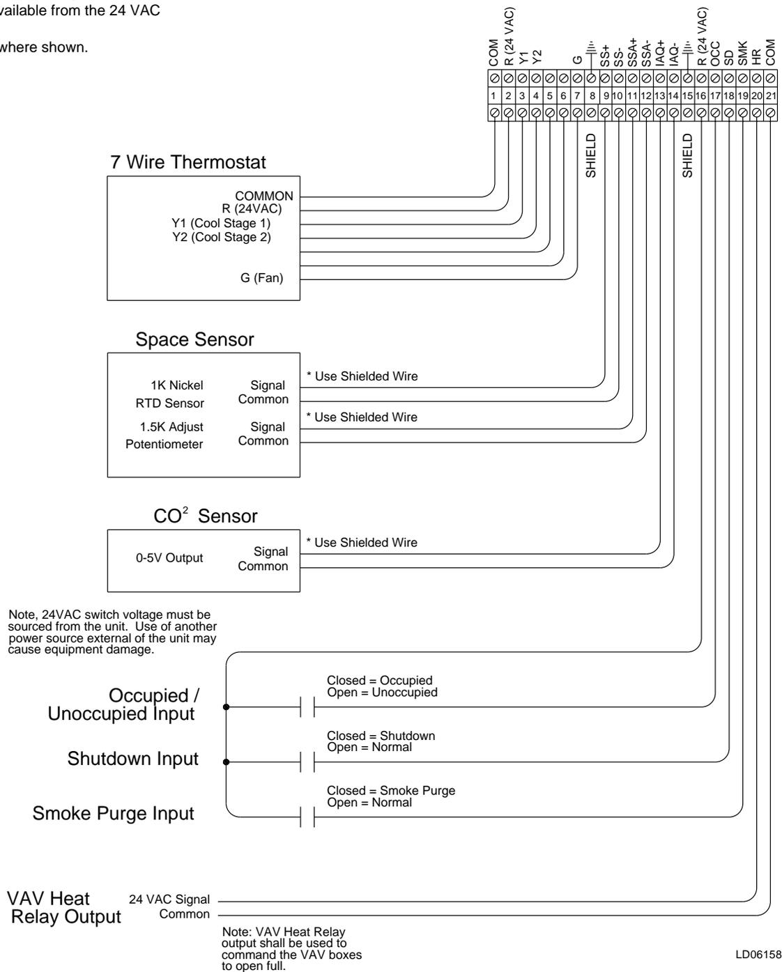
FIG. 5 – FIELD CONTROL WIRING
