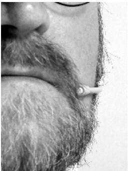
INCORRECT POSITIONING OF THE MICROPHONE FIGURE 6
