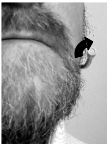
“ROLLING” THE MICROPHONE BOOM FIGURE 7
