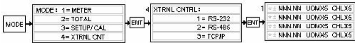
Press the **MODE** button. The **MODE** menu is displayed. Press the number “4” key for **XTRNL CNTRL**. The **XTRNL CNTRL** menu is displayed. Choose RS-232 by pressing the number “1” key. The normal display will return to its previously programmed state.
