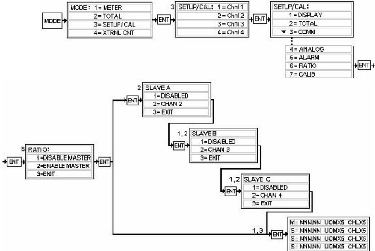
Press the **MODE** key and then **3 + ENTER**. Select channel one by pressing **1 + ENTER**. Choose **RATIO** by pressing the **6** key + **ENTER**. Channel one (1) is enabled as the master when you press **2 + ENTER**.
