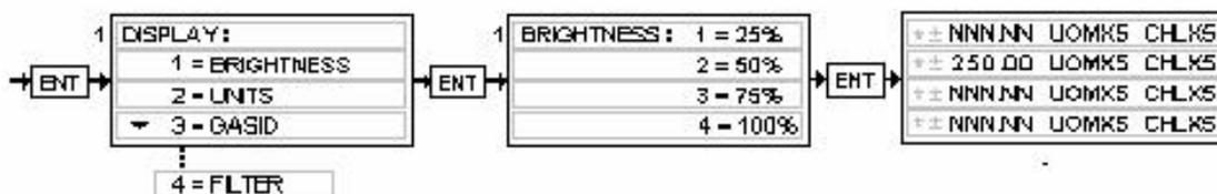
While the **SETUP/CAL** menu is displayed, choose **DISPLAY** by pressing the keys “1” + **ENTER**. Choose **BRIGHTNESS** by pressing the number “1” key + **ENTER**. The **BRIGHTNESS** menu will be visible. One of four different brightness levels can be chosen by pressing a number key. The number “1” key selects the dimmest setting while the number “4” key selects the brightest. Any change in brightness will affect the entire display after pressing the **ENTER** key.
