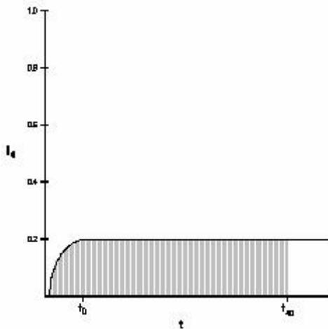
Each channel samples the incoming signal at a rate corresponding to the preset A/D conversion rate in Hz. At each sampling interval, the TOTALIZER function multiplies the average signal, as a fraction of the full-scale value (5v, 10v or 20 mA), times the *span*, or *cal*, value. This results in a rate for that interval. Next, a time element factor is determined according to the flow rate programmed for that channel as follows.
