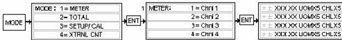
Press the **MODE** key. The **MODE** menu appears in the display. To select **METER**, press **1**, and then **ENTER**. The **METER** menu allows the selection of the desired channel. Press the number key that corresponds with the desired channel followed by **ENTER**. The previously programmed display returns with the selected channel reading the signal between pins 5 and 6 of the corresponding channel's 15 pin D-connector (J1 – J4).
