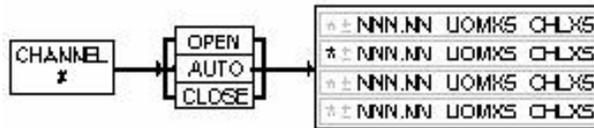
Press the desired **CHANNEL #** key. An asterisk appears in the first space on the line representing the selected channel. The meter display is immediately replaced with the current set point. Pressing the **AUTO** key causes pin number eight (8) of the 15 pin Sub-D connector to float and returns the previously programmed metering function to the display. Pin 14 signal levels are now available for control.
