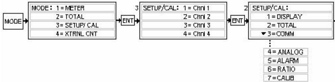
Pressing the **MODE** key causes the **MODE** menu to be displayed. Choose the **SETUP/CAL** mode by pressing the number “3” key then **ENTER**. A **CHANNEL SELECT** menu is presented on the display. It should be noted that, although the user must select a specific channel number, some choices in the following menus may affect the operation of all channels and/or the display (ex; Display Brightness, type of communication). See the following menu options for more details.
