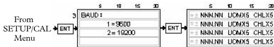
After selecting **SETUP/CAL**, select any channel number and hit **ENTER**, choose option number **3** via the numbered key pad. The **BAUD** menu will be displayed. To select the desired baud rate press the corresponding number key.
