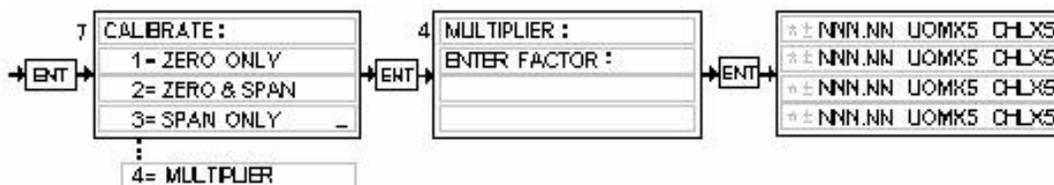
For convenience, it is possible to leave a channel setup one way and merely multiply the display value by some factor and replace the display with the new value. An example might be to set up a channel to read from zero to one hundred percent and use a multiplication factor to make the display read from zero to 500 SCCM. An infinite number of possibilities are possible.
