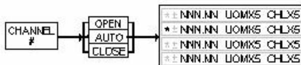
Press the desired **CHANNEL #** key. An asterisk appears in the first space on the line representing the selected channel. The meter display is immediately replaced with the current set point. Pressing the **CLOSE** key results in the application of -15 VDC to pin number eight (8) of the corresponding 15 pin Sub-D connector and returns the previously programmed metering function to the display.
