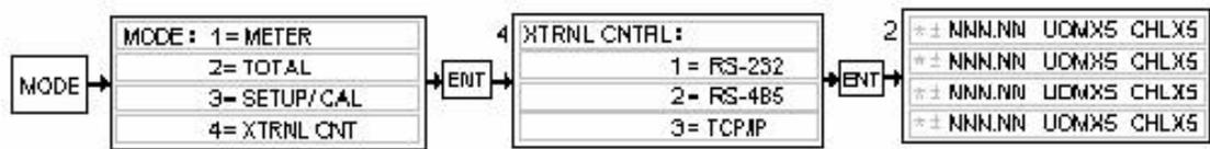
Press the **MODE** button. The **MODE** menu is displayed. Press the number “4” key for **XTRNL CNTRL**. The **XTRNL CNTRL** menu is displayed. Choose RS-485 by pressing the number “2” key. The normal display will return to its previously programmed state.
