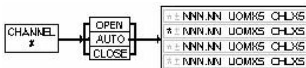
Press the desired **CHANNEL #** key. An asterisk appears in the first space on the line representing the selected channel. The meter display is immediately replaced with the current set point. Pressing the **OPEN** key results in the application of +15 VDC to pin number eight (8) of the corresponding 15 pin Sub-D connector and returns the previously programmed metering function to the display.
