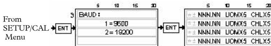
After selecting **SETUP/CAL**, select any channel number and hit **ENTER**, choose option number **3** via the numbered key pad. The first menu to be displayed is the **BAUD** menu. To select the desired baud rate press the number key **1** or **2** respectively. Eight bit bytes, no parity, one stop bit and no handshaking are automatically set. The preprogrammed display is returned upon completion.
