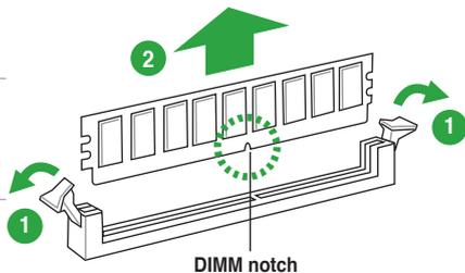
2. Remove the DIMM from the socket.
