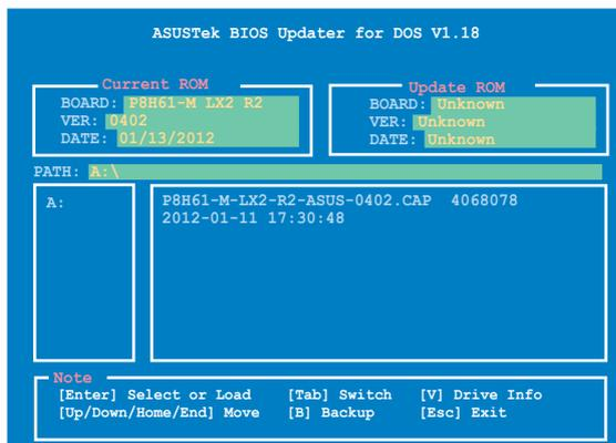
3. Press <Tab> to switch between screen fields and use the <Up/Down/Home/End> keys to select the BIOS file and press <Enter>. BIOS Updater checks the selected BIOS file and prompts you to confirm BIOS update.
