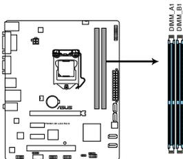
P8H61-M LX2 R2.0 240-pin DDR3 DIMM sockets
