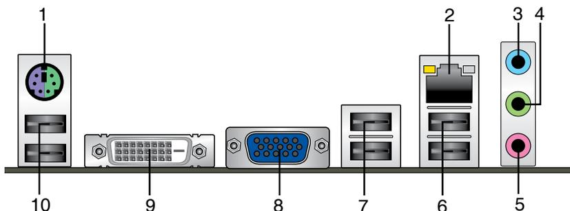
1. **PS/2 Keyboard / Mouse Combo port.** This port is for a PS/2 keyboard or PS/2 mouse.
