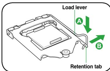
3. Lift the load lever in the direction of the arrow until the load plate is completely lifted.
