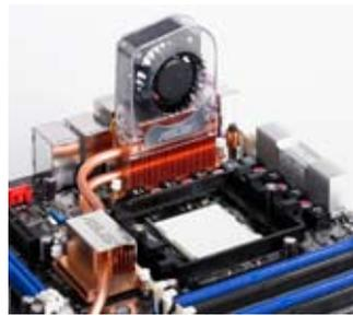
4. The above photo shows the fans installed on the motherboard.
