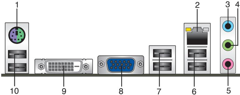
1. **PS/2 keyboard/mouse combo port.** This port is for a PS/2 keyboard/mouse.
