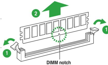
2. Remove the DIMM from the socket.
