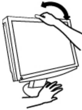
**(3) If necessary, fine adjust the height of the monitor.**
