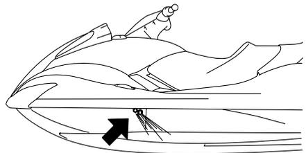
To check for proper operation of the cooling system, check that water is being discharged from the port (left) pilot outlets. If water is not being discharged from these outlets, cooling water may not be circulating in the engine. When this occurs, stop the engine and check
