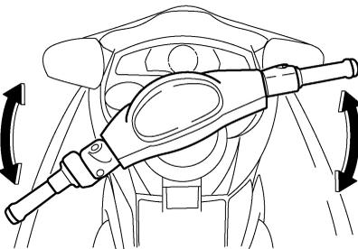
Push the handlebars back and forth to check that the tilt lever and handlebars are locked in
