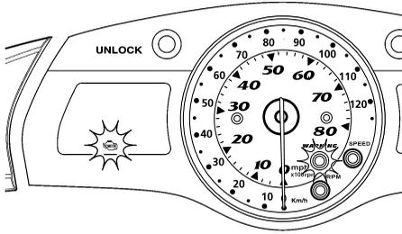
If this occurs, reduce the engine speed, return to shore, and have a Yamaha dealer check the engine.
