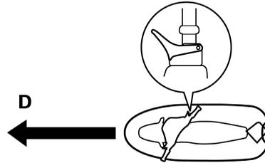
C. Releasing the throttle lever completely produces only minimum thrust. If you are traveling at speeds above trolling, you will have rapidly decreasing ability to steer without throttle. You may still have some turning ability immediately after releasing the throttle lever, but once the engine slows down, the watercraft will no longer respond to handlebar input until you apply throttle again or you reach trolling speed.
