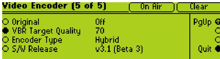
When running in VBR Mode the two top-level status screens show the current bit-rate being used. This will typically vary.
