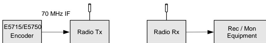
Figure 1.6: Typical DENG System Configuration
