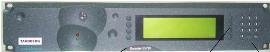
Each softkey on each side of the display is used to access, select and sometimes amend the menu item associated with it.
