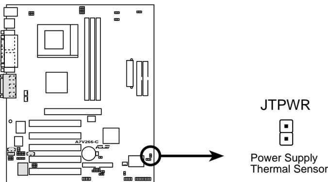
**A7V266-C Thermal Sensor Connector**
