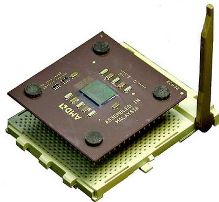
3. Once completely inserted, press the CPU firmly and close the socket lever until it snaps into its locked position.
