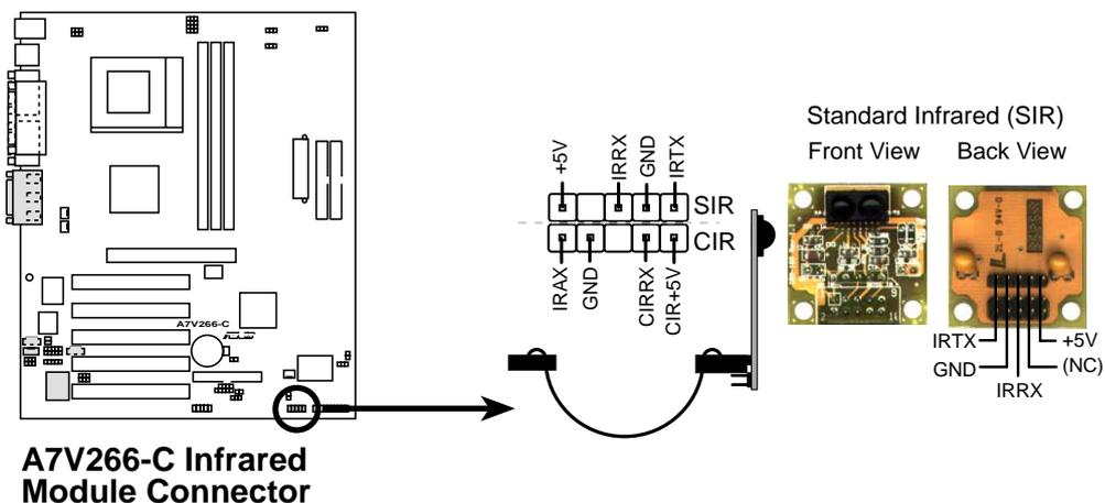
**A7V266-C Infrared Module Connector**
