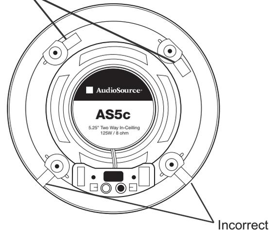
With the grill removed, place the speaker in the ceiling opening. Make sure that the speaker wire is not hanging against the speaker where it can vibrate and rattle as the speaker reproduces your audio program.
