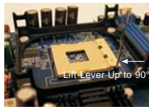
STEP 1: Lift The Socket Lever Up to 90°
