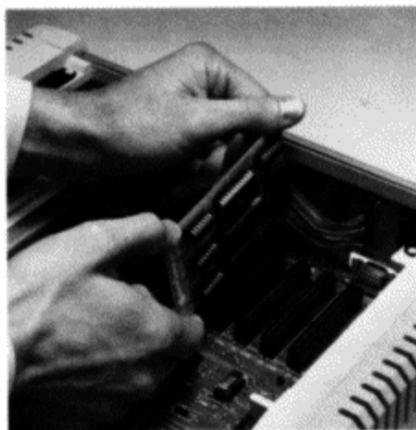
Figure 8. Installing the Interface Card in an Apple IIe
