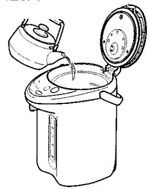
● If water of approx. 122°F or greater is poured, the automatic heating will not commence. Therefore, if this is the case, add some warm water or just water. Otherwise, you can press the Re-boil key. (For the re-boiling procedures, see page 23.)
