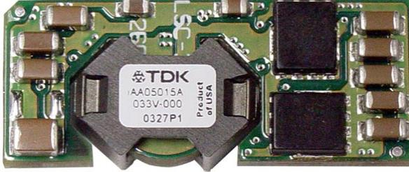
The Metamere Series offers a 50W power module in the industry's standard surface-mount footprint. The Metamere series utilizes a low component count that results in a low cost while still providing high performance. The open-frame, compact design provides flexibility by performing local voltage conversion of either a 5V or 3.3V bus. The low weight, surface mount design is well suited for almost any manufacturing environment.
