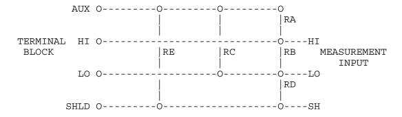
RA, RB, RC, RD and RE are selected separately for each input and are labeled on the PC board for each loop. CH 1 (channel 1) is loop 1 etc. Resistors should be 0.1% metal film, 1/4 watt. Other components such as
