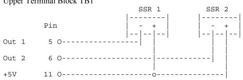
Alarm outputs are also used to activate SSR's when possible. The connections are essentially the same.
