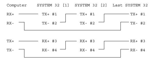
Multiple SYSTEM 32 units are connected in series. R+ is connected to the first unit TX+ and TX- from the first unit is connected to TX+ of the next unit. These serial connections are continued until the last unit is reached. The last unit TX- is connected to the computer R-. T+ is connected to the first unit RX+ and the RX- is connected to the next unit RX+. The last unit RX- is connected to the computer T-.
