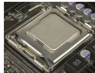
Align notches with notches on the CPU
