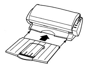
2) Hold the document support and insert its tabs into the counterpart holes on the scanner as shown in the figure below.
