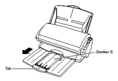
2) Insert a finger into the dent at the center of the stacker, then lift and pull the Stacker B.
