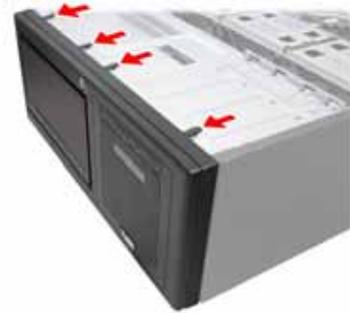
2. Remove the door assembly from the four holes located on the lower edge of the server.
