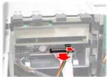
3. Unfasten the installed drives or the empty drive brackets from the chassis in the direction of the arrow shown.
