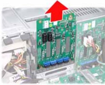
5. Place a new backplane in position and secure in place with one screw.
