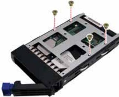
5. Insert the drive tray back into the chassis and push the locking lever into place to secure it.
