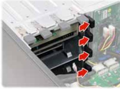
4. Slide all the drives or the brackets out of the chassis.
