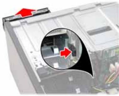
5. Use a thin tool such as a flat screwdriver to pry open the front panel of the drive bracket as indicated.
