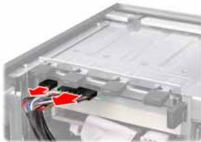
3. Unfasten the LED module and slide it out as shown to lift it free of the chassis.
