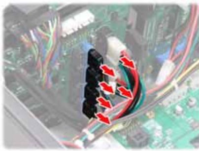
9. Connect the other end of the SATA/SAS cables to the connectors on the PCI-E RAID card.
