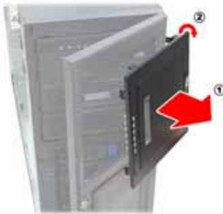
8. Fit the front bezel back into position.
