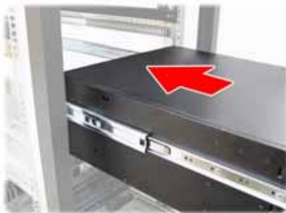
10. Push the unit in and press the latch key.
