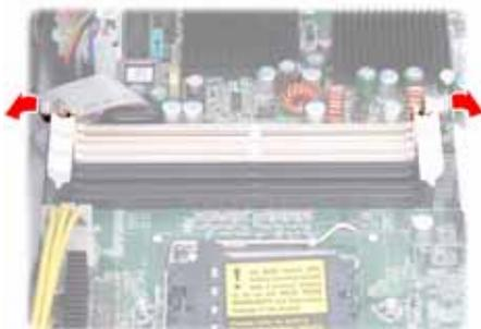
4. Align the memory module with the slot. The module has indentations that align with notches in the slots.
