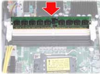
When inserted properly, the memory slot locking levers lock automatically onto the indentations at the ends of the module.
