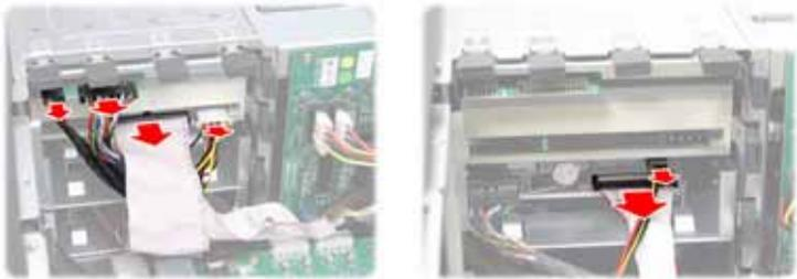
2. Unfasten the installed drives or the empty drive brackets from the chassis in the direction of the arrow shown.
