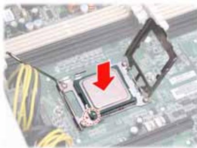
**NOTE:** The CPU will only fit in the socket one way. No force should be required to insert the CPU.
