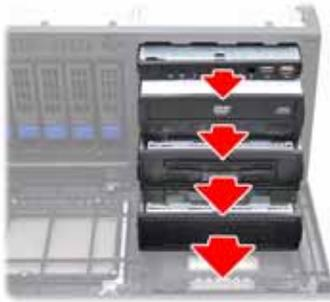
5. Slide all the drives or the brackets back into the chassis vertically.
