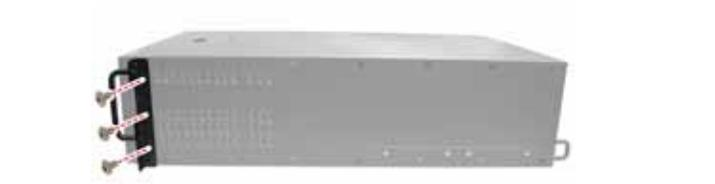
3. Draw out the inner rails from each rail assembly. Install the inner sliding rails to each side of the server using five M4-L5 screws (C).
