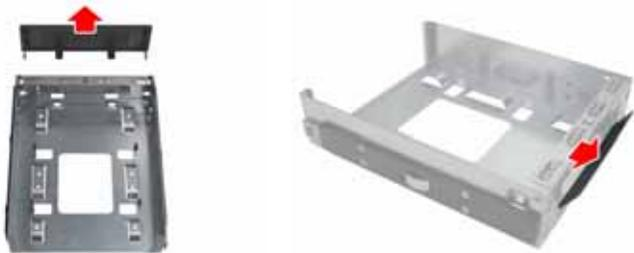
7. Install the FDD front panel to the front of the bracket.
