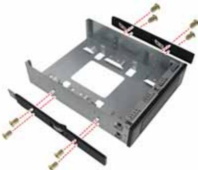
4. Attach the two rails removed from the drive bracket to the DVD-ROM with eight screws.
