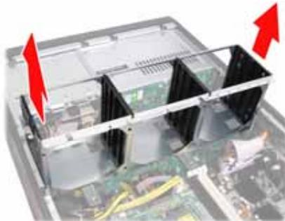
4. Unfasten an empty drive bracket from the chassis in the direction of the arrow shown.
