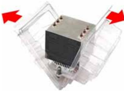
9. Place the fan and heatsink on top of the CPU and attach with two screws as shown.
