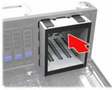
11. Install the SAS or SATA hard drives in the drive trays as instructed in the previous section.
