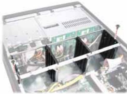
3. Remove the fan cradle as instructed to reveal the fan control board.
