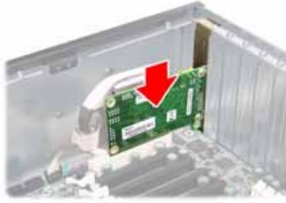
6. Secure the PCI bracket with the screw you removed from the blanking plate.
