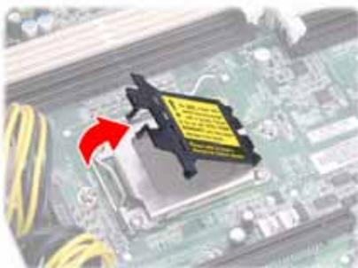
4. Lift up the CPU lever to unlock the socket.
