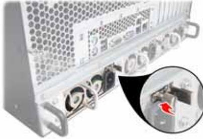
2. Press the latch and the handle together as shown.
