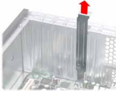
4. Insert a PCI-E/PCI card into an appropriate slot, making sure it is firmly seated. Secure it with the screw removed in step 2.
