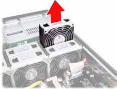
2. Replace a new fan into the fan cradle following the above steps in reverse.
