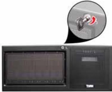
2. Pull the front bezel in the direction of the arrow to open.
