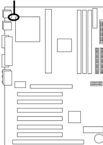
**Warning: If JP21 is set to the incorrect CPU type, there will be no video display at Post. Please correct the jumper setting and reboot the system.**
