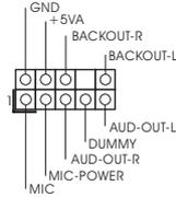
This is an interface for the front panel audio cable that allows convenient connection and control of audio devices.
