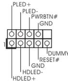
This connector accommodates several system front panel functions.
