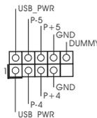
ASRock I/O™ provides you four default USB 2.0 ports on the rear panel. If the USB 2.0 ports on the rear panel are not sufficient, you may use this USB 2.0 header to attach two additional USB 2.0 ports.
