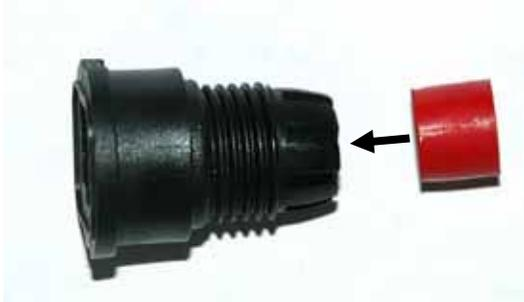
2. Strip the CATx shielded cable jacket (6mm-7mm O.D.) approximately 1/2" and insert the cable through the sealing nut, screw nut, and housing. (Note: Heat shrink tubing can be applied to cable to increase the O.D. to 6mm-7mm.)
