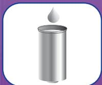
Dosing of electrolyte into separator with subsequent time for soaking.
