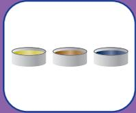
Manganese dioxide, graphite, binder and alkaline electrolyte are mixed and consolidated into rings.
