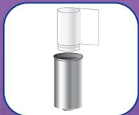
The widened edge is coated. Insertion of the wound separator and bottom cup.
