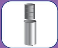
Ring insertion into the can. Recompaction of the rings into the can.
