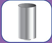
Can production by deep drawing in several steps. The can surface will be coated with graphite.
