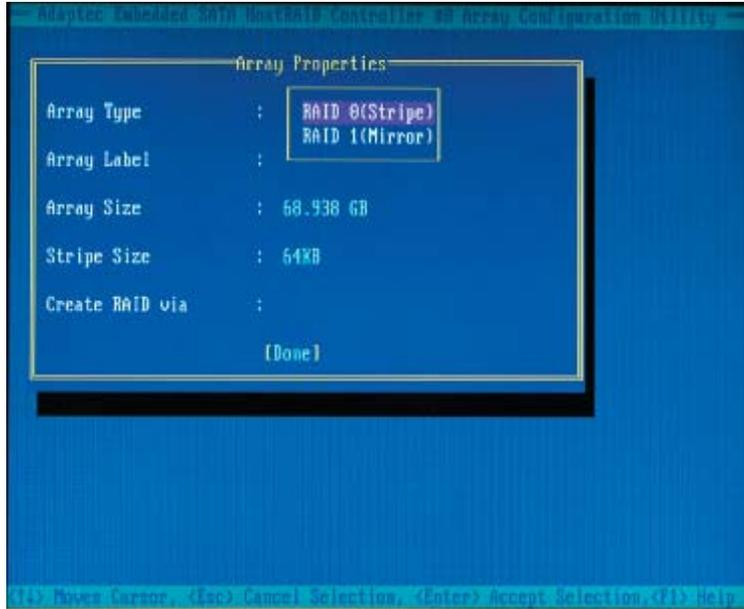
2. Under the item "**Arrays Label**", type in a label and press <Enter>. (\*Note: The label shall not be more than 15 characters.)
