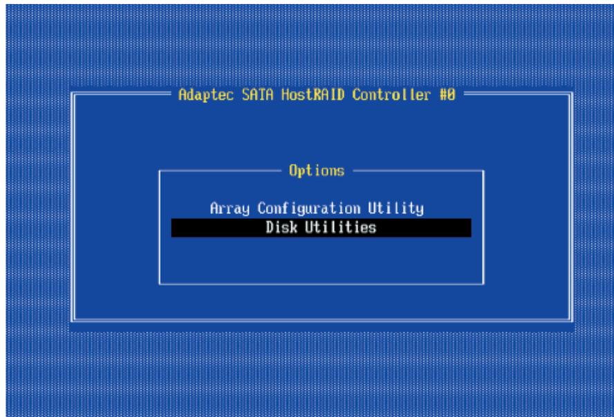
1. From the Adaptec RAID Configuration Utility Menu, select **Disk Utilities** (as shown above) and press **<Enter>**. The following screen appears.
