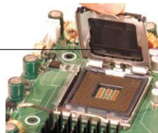
3. Use your thumb and your index finger to hold the CPU at the North Center Edge and the South Center Edge of the CPU.
