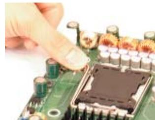
2. Gently lift the socket clip to open the load plate.
