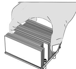
3. Once the CPU is loosened, remove the heatsink from the CPU socket.
