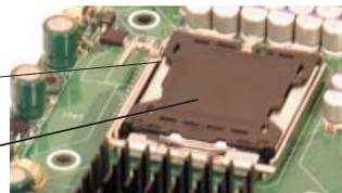
1. Press the socket clip to release the load plate, which covers the CPU socket, from its locking position.
