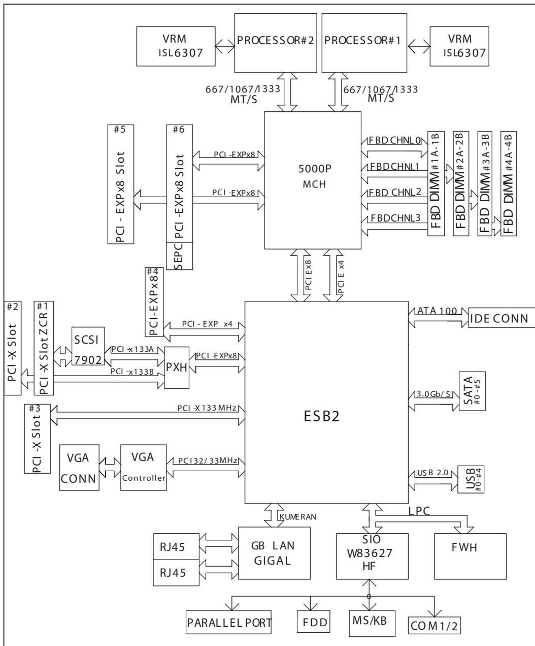
Figure 1-9. Block Diagram of the 5000P (Blackford) Chipset
