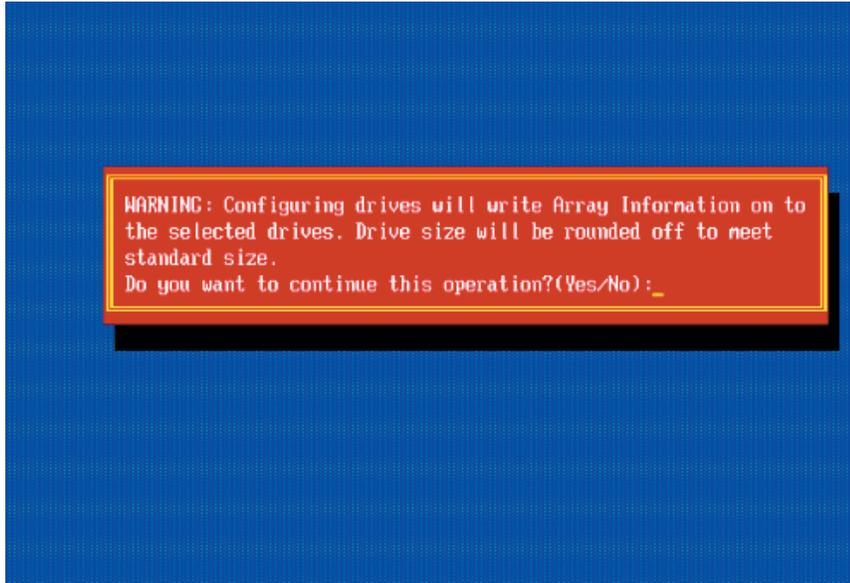
6. Make sure that you have selected the correct disk drives to configure. If correct, type **Y** to continue.
