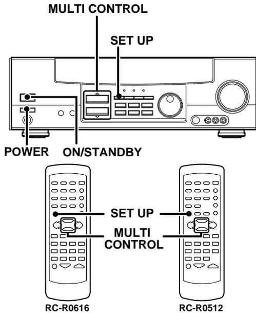
**1** Turn on the power to this receiver by pressing **POWER** or **ON/STANDBY** key.
