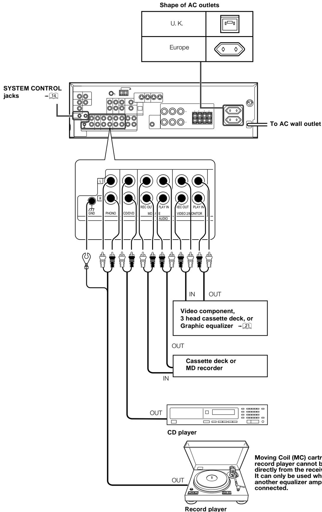
When you connect the audio cord of the video component to the VIDEO2/ MONITOR jacks, connect the video cord (yellow RCA pin cords) of the connected component to the VIDEO2 IN jack.
