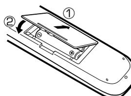
• Insert two AA-size (R6) batteries as indicated by the polarity markings.
