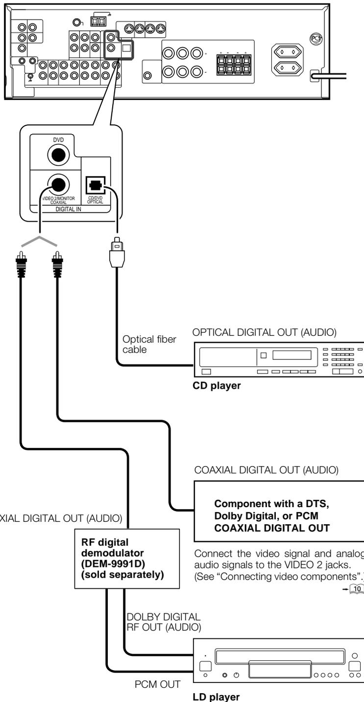
To connect an LD player with a DIGITAL RF OUT, connect the LD player to the KENWOOD RF digital demodulator (DEM-9991D). Next, connect the DIGITAL OUT jacks of the demodulator to the DIGITAL IN jacks of the receiver. Connect the video signal and analog audio signals to the VIDEO2/MONITOR jacks. (See "Connecting video components".)
