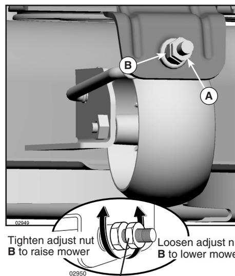
Tighten adjust nut B to raise mower
