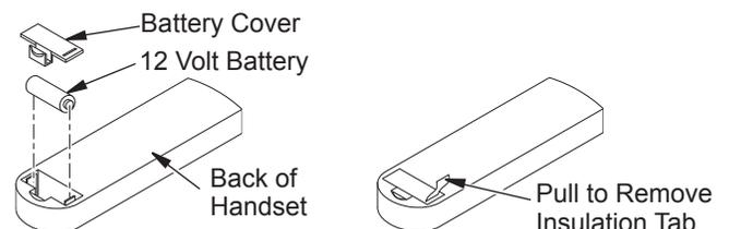
Figure 41 - Installing Battery into Back of Handset
