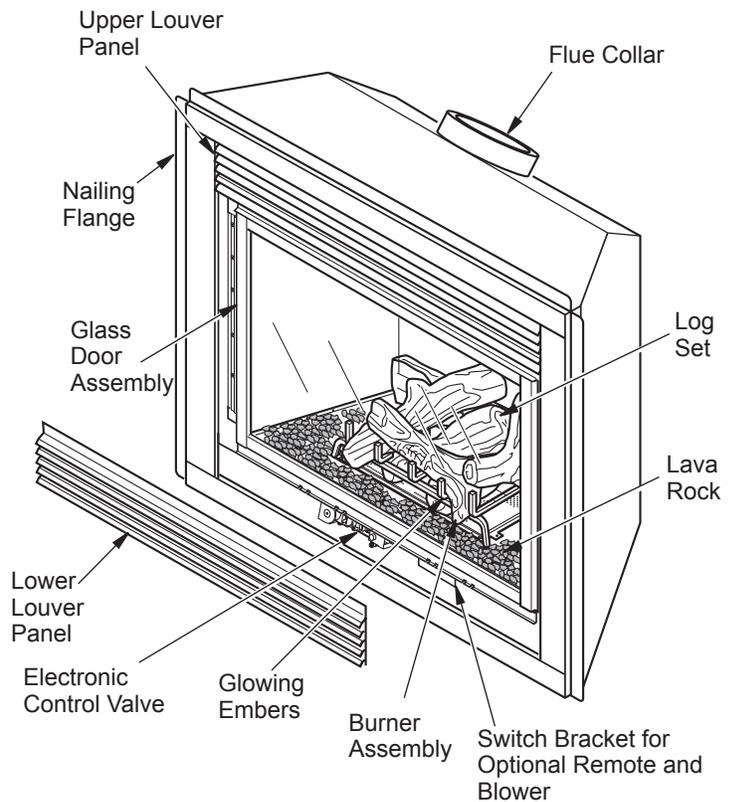
Figure 1 - Direct-Vent Fireplace with Electronic Ignition
