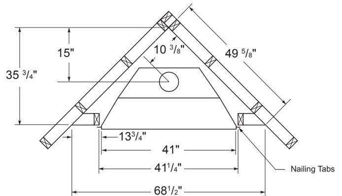
Figure 5 - Framing Clearances for Corner Installation
