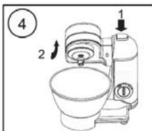
3. Insert desired attachment onto "Attachment Post" (4) and press upward as far as possible. (Fig.5)
