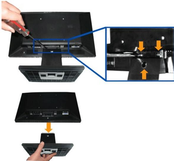
To remove the stand assembly from the monitor:
