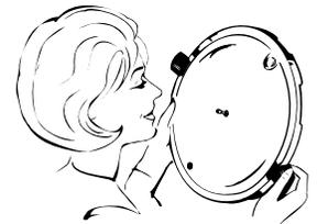
6. Place cover on canner, aligning the V mark on the cover with the A mark on the body handle and lock securely by turning in the direction indicated to close (clockwise). **Cover handles must be centered over body handles. Do not force beyond this position.**
