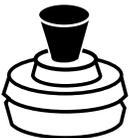
The pressure regulator controls and maintains the correct pressure in the canner. The correct pressure is obtained when the pressure regulator begins a gentle rocking motion.
