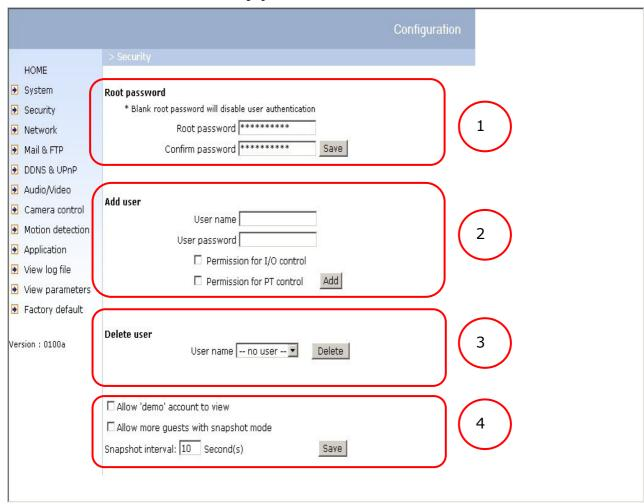
Network Camera is shipped without any password by default. That means everyone can access Network Camera including the configuration as long as the IP address is known. It is necessary to assign a password if the Network Camera is intended to be accessed by others. Type a new word twice in ① to enable protection. This password is used to identify the administrator. Then add an account with user name and password for your friends in ②. Network Camera can provide twenty accounts for your
