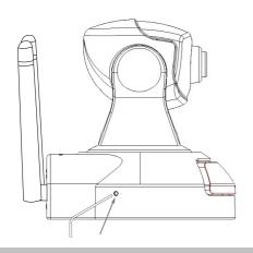
Restoring the factory defaults will erase any previous settings. Reset or restore the system after power on.
