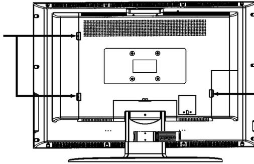
Before you connect external devices with the unit, please remove the Back Cover first.
