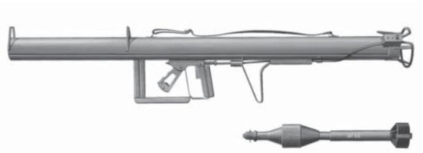
**Operation** Rocket launcher, electrically fired
