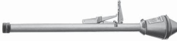
**Operation** Grenade launcher, percussion fired
