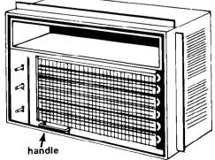
**5.** Pull out wire handle at bottom and slide air conditioner unit out of cabinet.
