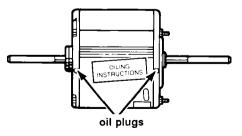
**10.** Oil the fan motor as instructed on the motor. Remove the oil hole plug at each end of the motor to add oil. An easy-to-use oil capsule is available from local service centers or you can use SAE #20 nondetergent oil. Replace plugs into each end of the motor.
