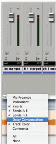
To view the latency introduced by plug-ins go to the bottom left hand corner of the Mix view, click on the small black/grey box and select 'Delay Compensation'.
