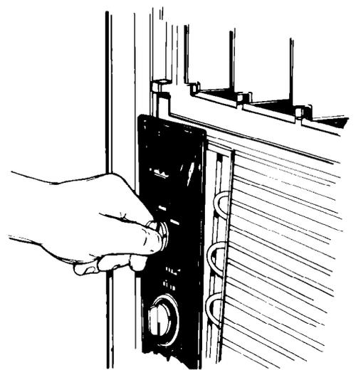
3. Pull control knobs straight off. Remove control panel.
