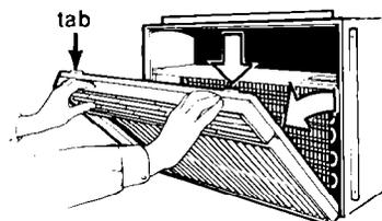
1. Press down on the top edge of front panel until it releases from the cabinet.
