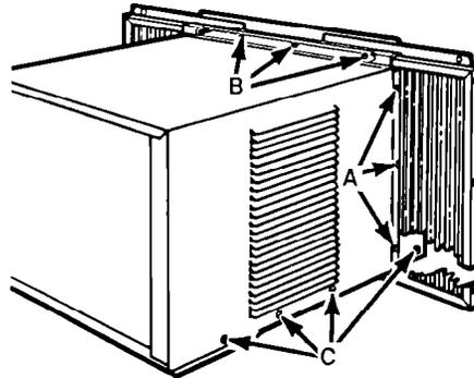
4. Slide curtains out to fullest width. Remove 6 Phillips-head screws that attach curtains to cabinet. (A)
