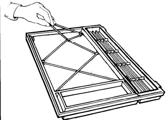
3. Remove elastic band from the back side of the front panel. Remove filter.
