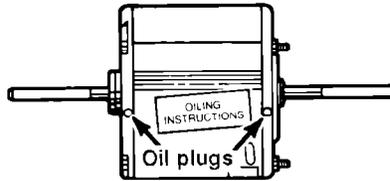
9. Oil the fan motor as instructed on the motor. Remove the oil hole plug at each end of the motor to add oil. An easy-to-use oil capsule is
