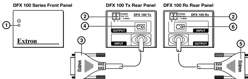
1. Connect one of the provided 12 VDC power supplies to the rear panel captive screw connectors of the transmitter and the other to the receiver (2).
