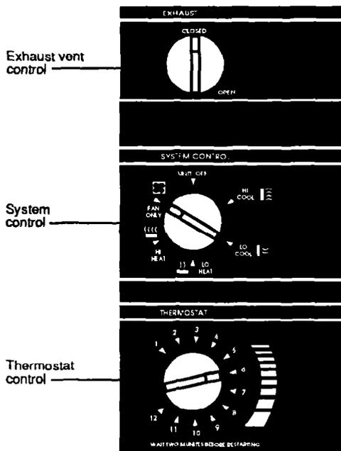
1. Set Exhaust Vent Control to CLOSED for maximum cooling.
