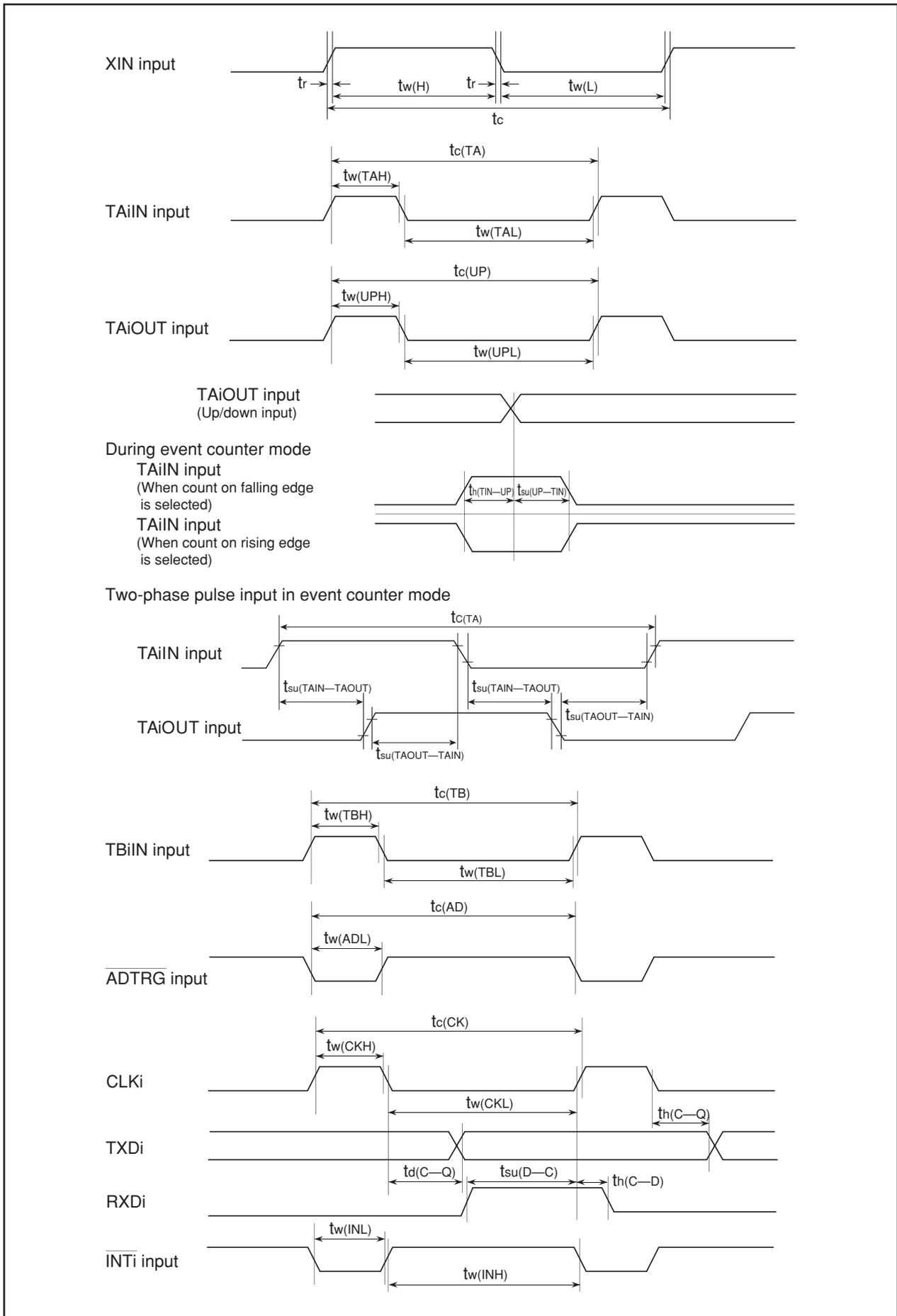
Figure 21.3 Timing Diagram
