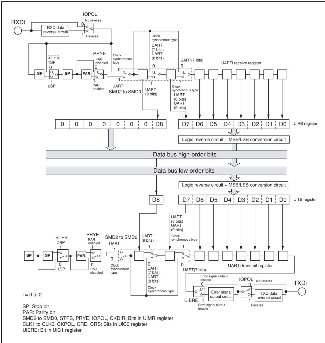
Figure 14.4 UARTi Transmit/Receive Unit
