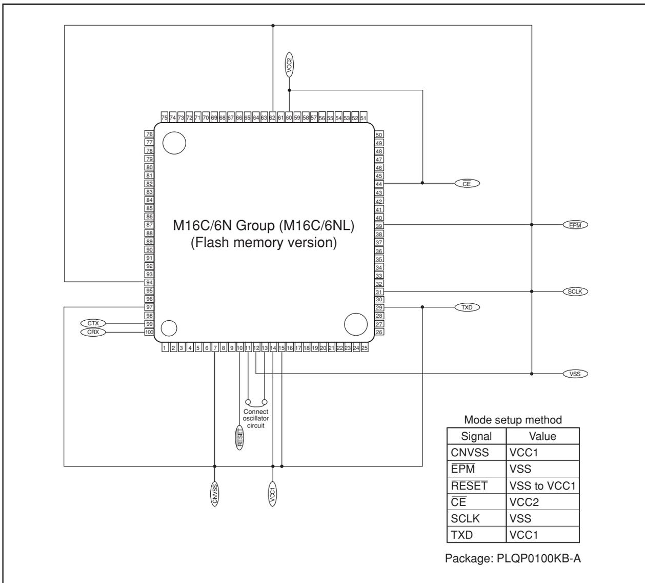
Figure 20.17 Pin Connections for CAN I/O Mode (1)
