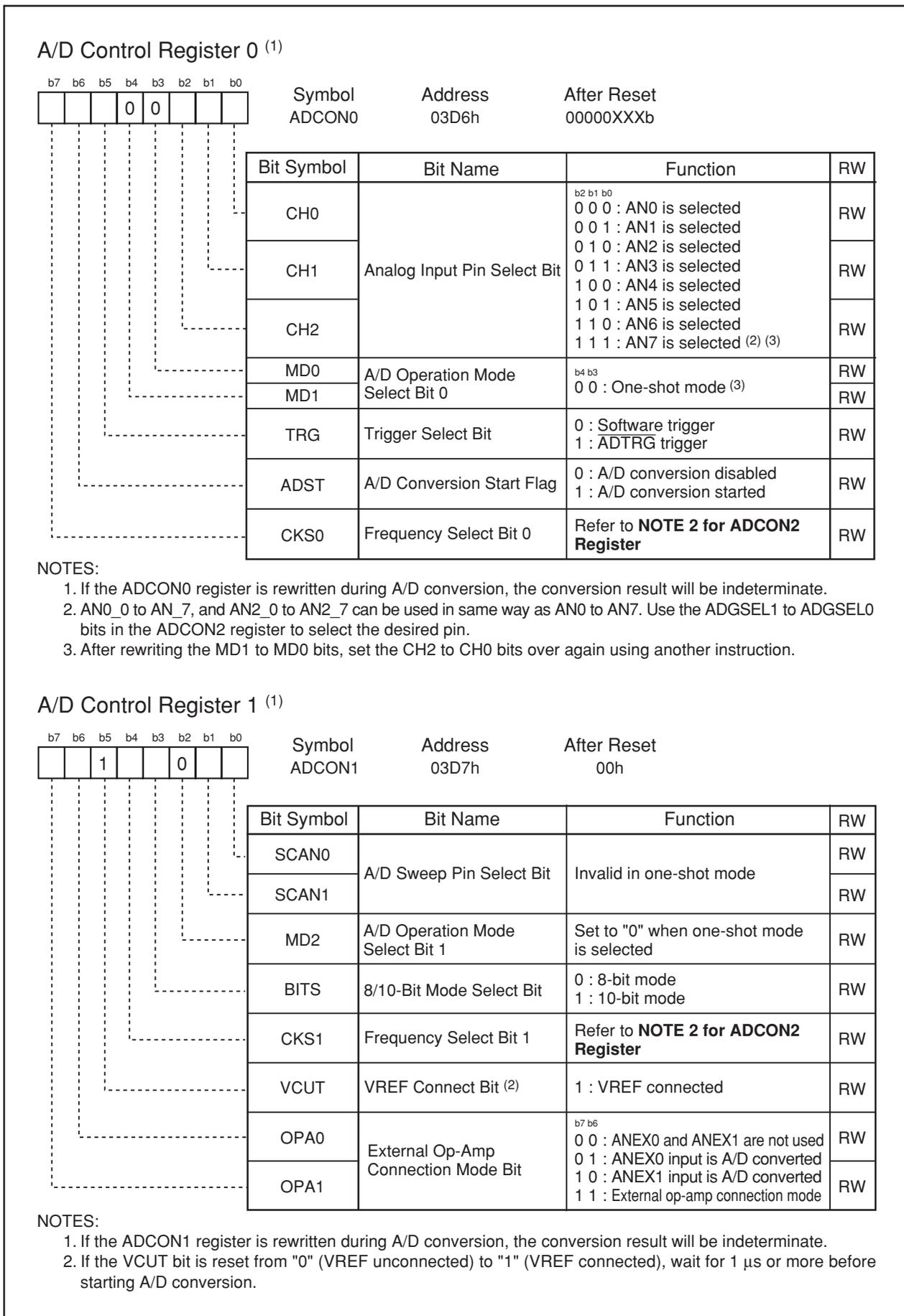
Figure 15.4 ADCON0 Register and ADCON1 Register in One-shot Mode
