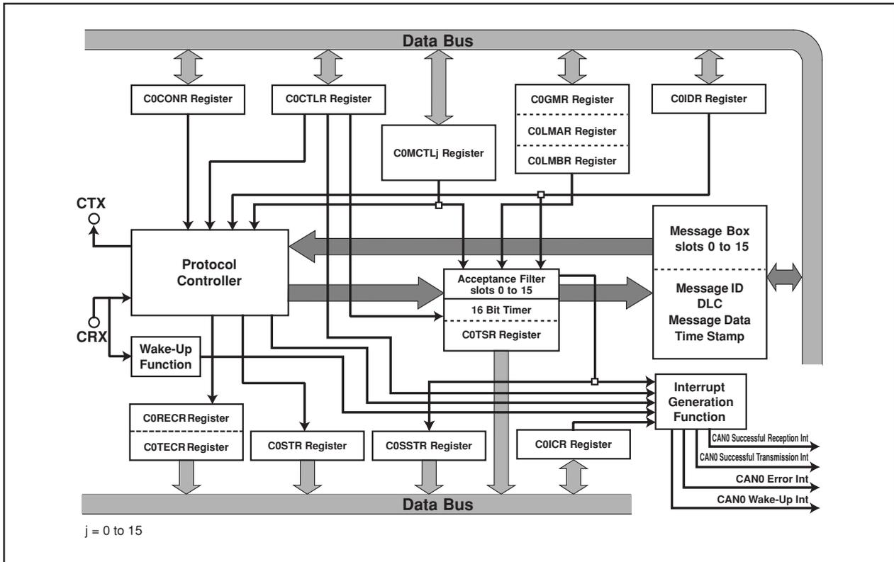
Figure 18.1 CAN Module Block Diagram
