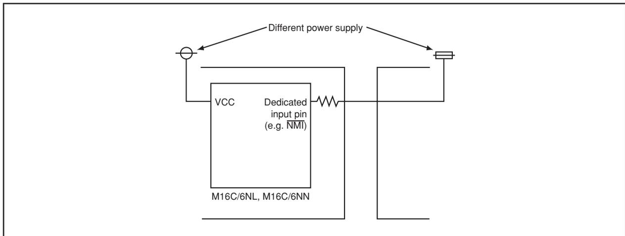
Figure 22.8 Circuit Connection
