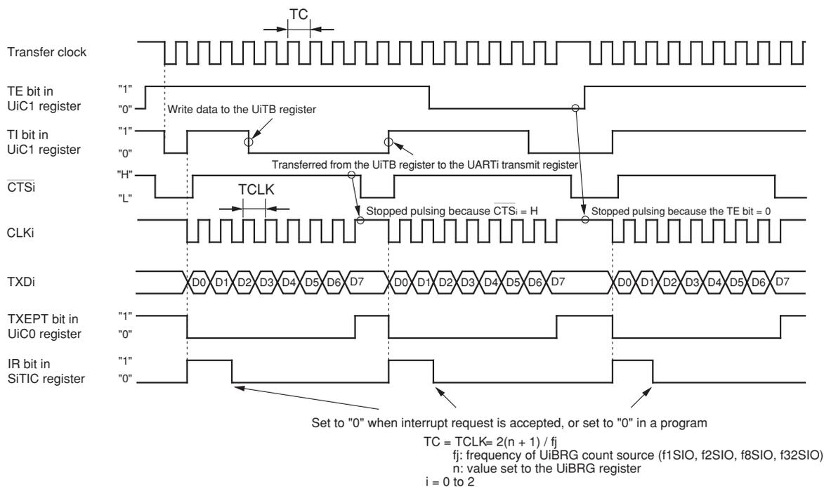
The above timing diagram applies to the case where the register bits are set as follows:
