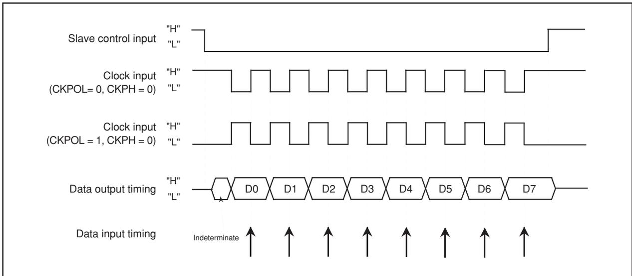
Figure 14.29 Transmission and Reception Timing (CKPH = 0) in Slave Mode (External Clock)
