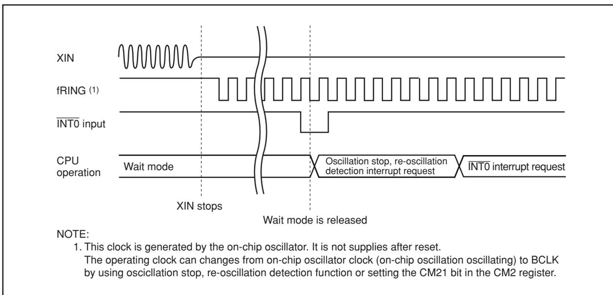
**Figure 22.1 Operation Timing at Oscillation Stop, Re-oscillation Stop Detection at Wait Mode (when moving out of wait mode by using INT0 interrupt)**
