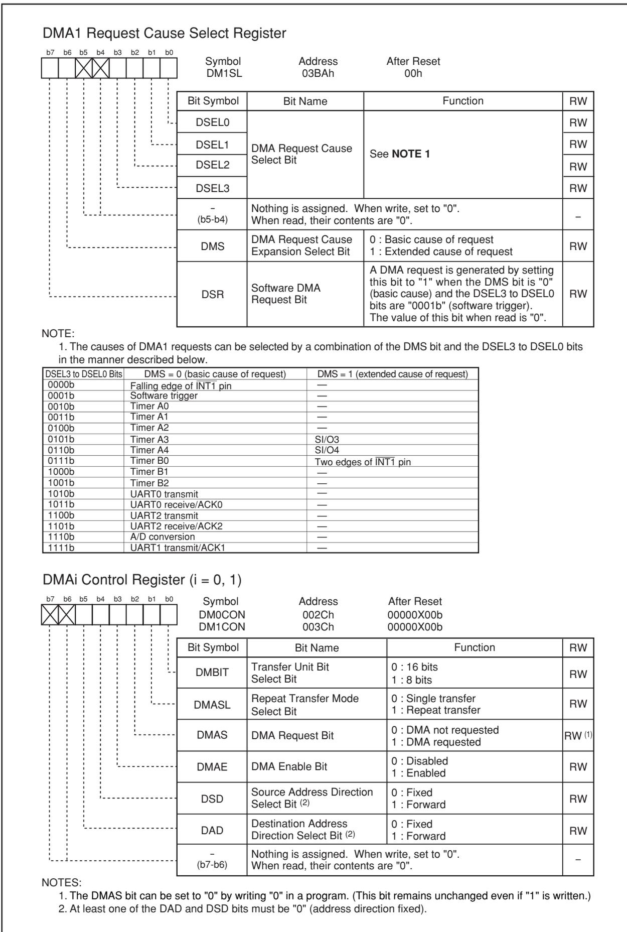
Figure 11.3 DM1SL Register, DM0CON and DM1CON Registers
