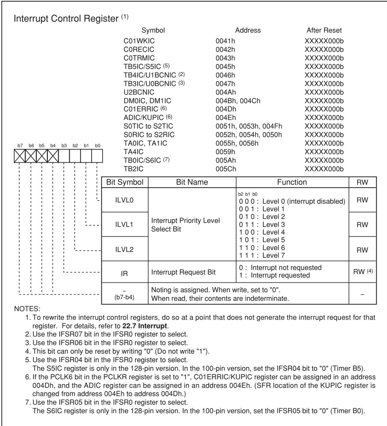
Figure 9.3 Interrupt Control Registers (1)
