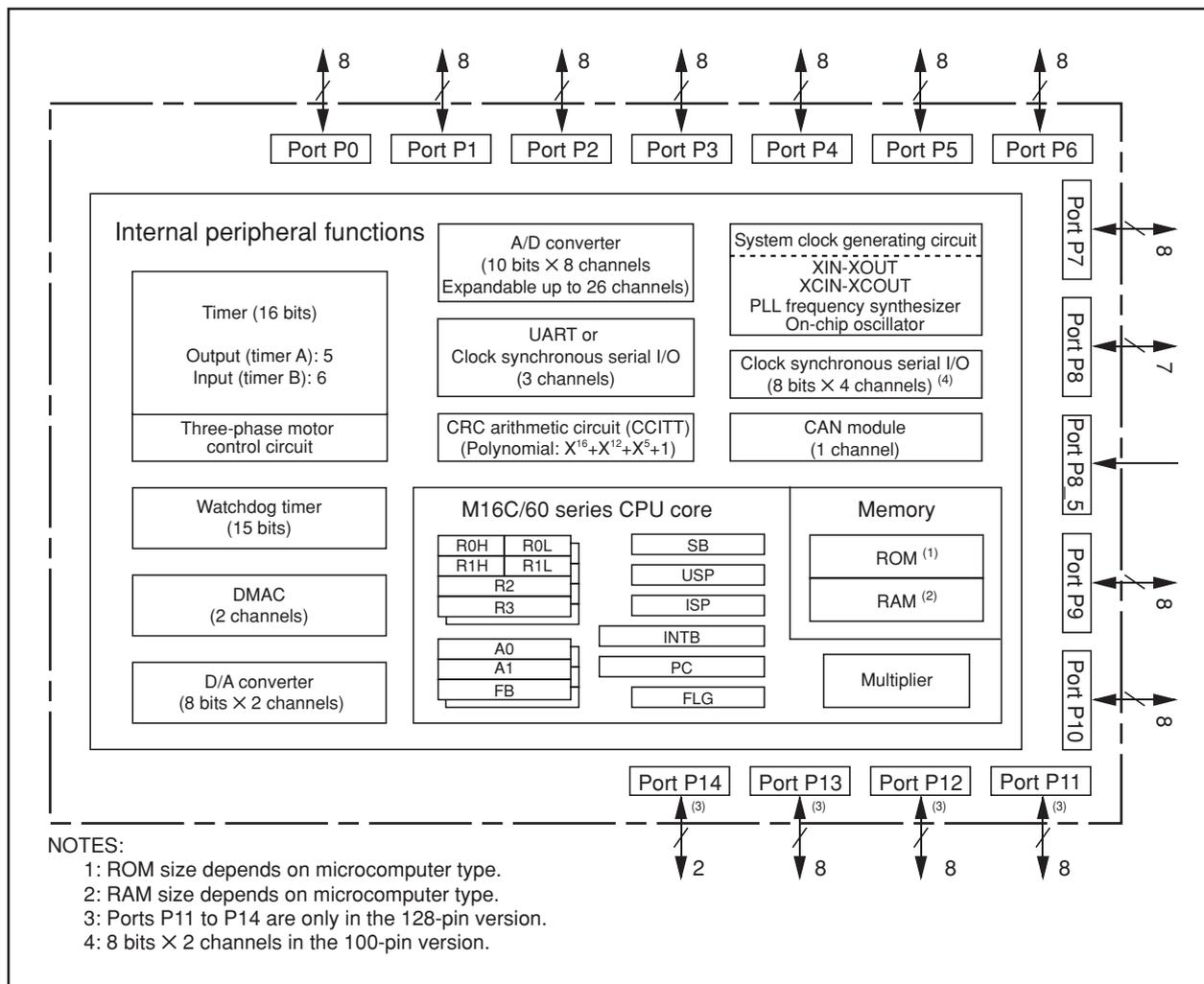
Figure 1.1 Block Diagram
