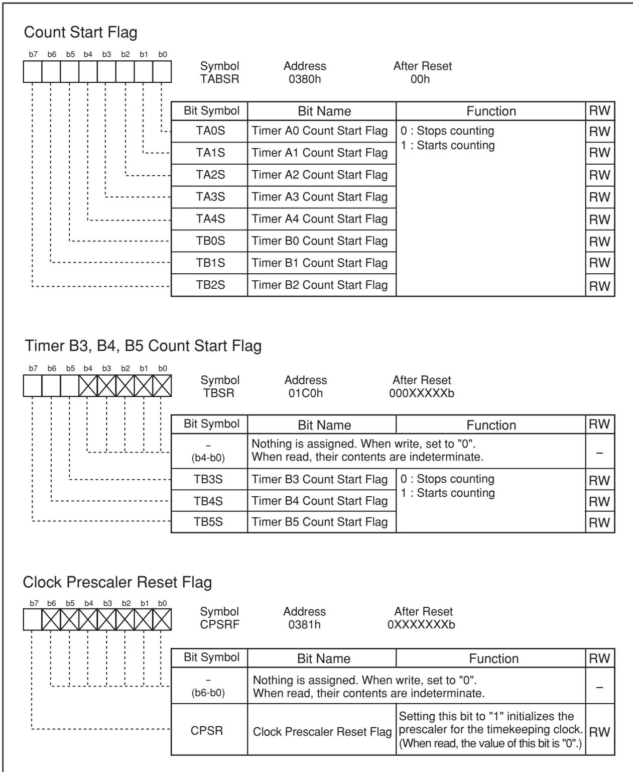
Figure 12.17 TABSR Register, TBSR Register and CPSRF Register
