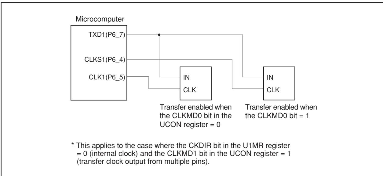
Figure 14.15 Transfer Clock Output From Multiple Pins
