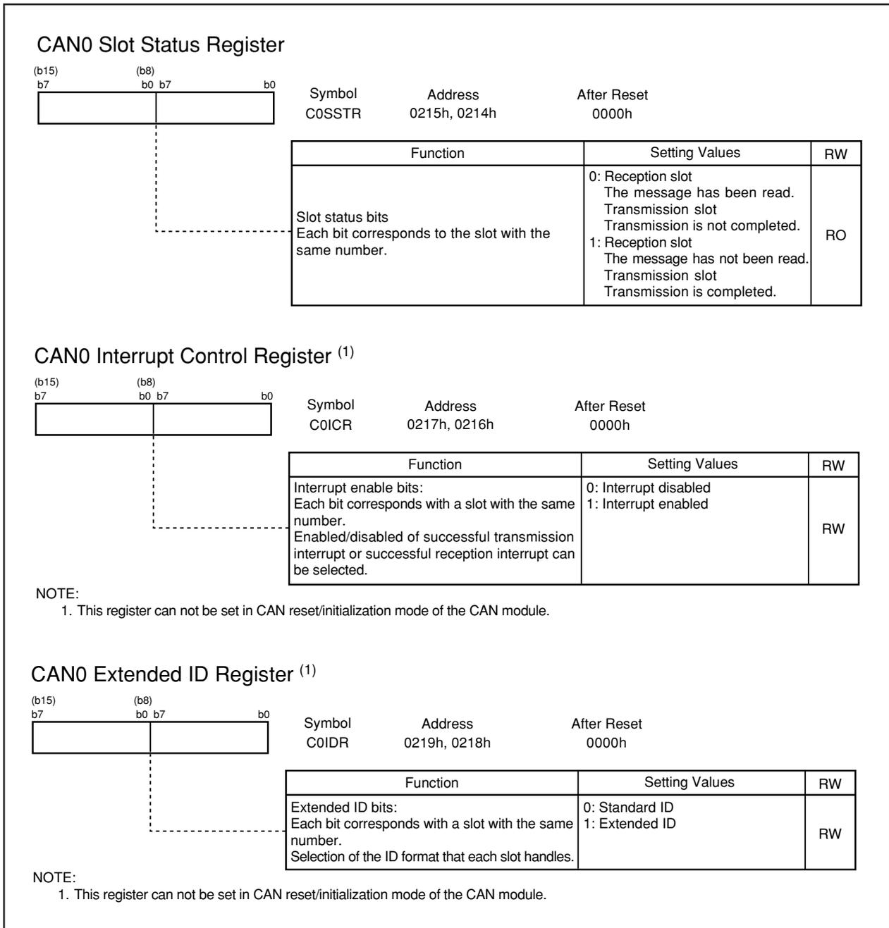
Figure 18.10 C0SSTR Register, C0ICR Register and C0IDR Register
