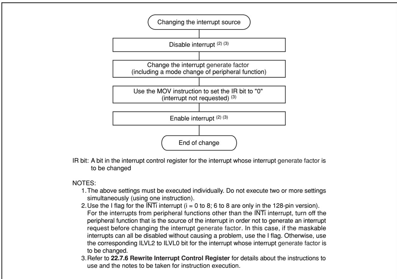
Figure 22.3 Procedure for Changing Interrupt Generate Factor
