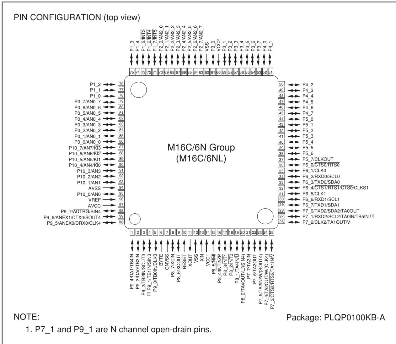
Figure 1.3 Pin Configuration (Top View) (1)
