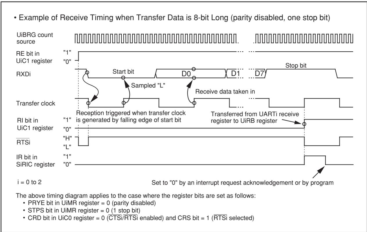
Figure 14.18 Receive Operation
