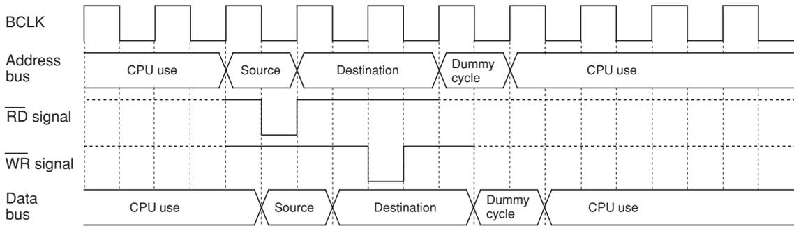
(2) When the transfer unit is 16 bits and the source address of transfer is an odd address, or when the transfer unit is 16 bits and an 8-bit bus is used
