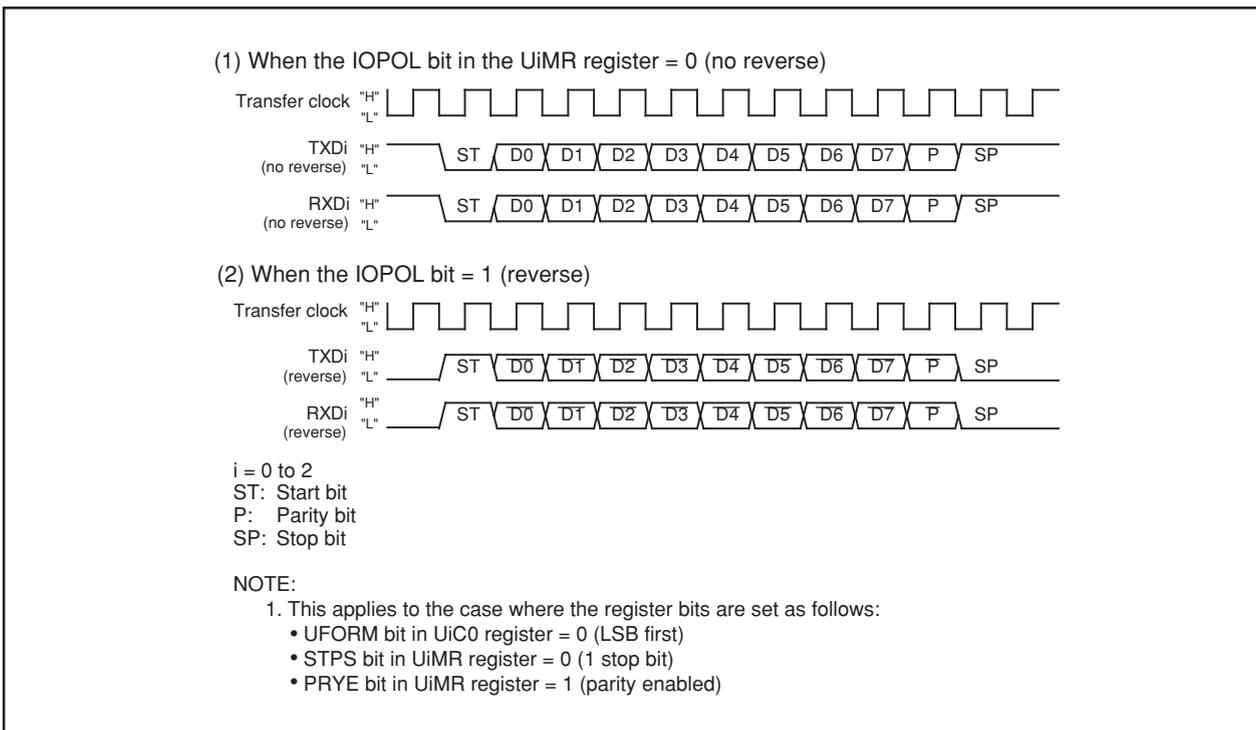
Figure 14.21 TXD and RXD I/O Polarity Inverse
