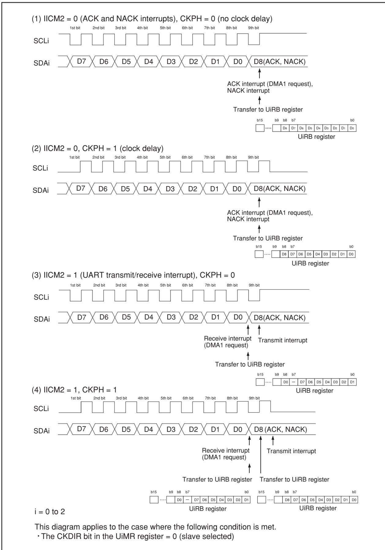
Figure 14.24 Transfer to UIRB Register and Interrupt Timing
