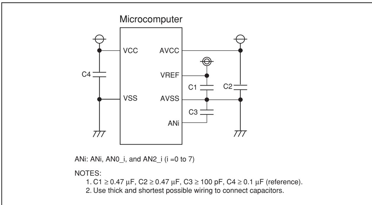
Figure 22.4 Use of Capacitors to Reduce Noise
