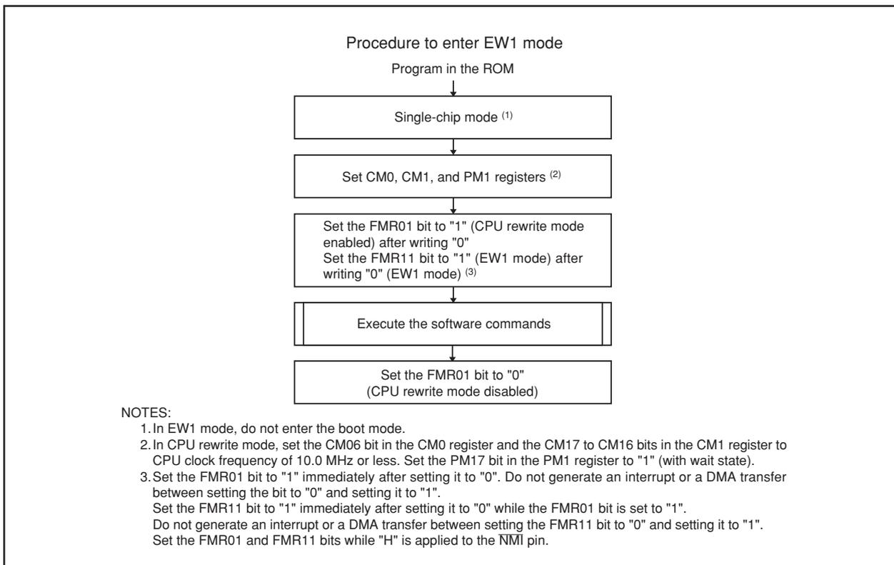
Figure 20.6 Setting and Resetting of EW1 Mode
