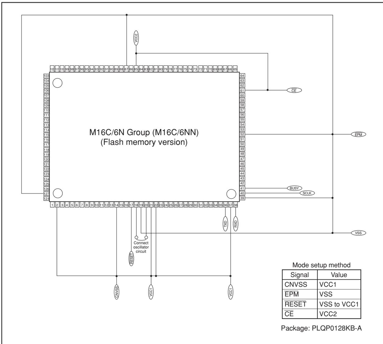
Figure 20.14 Pin Connections for Standard Serial I/O Mode (2)
