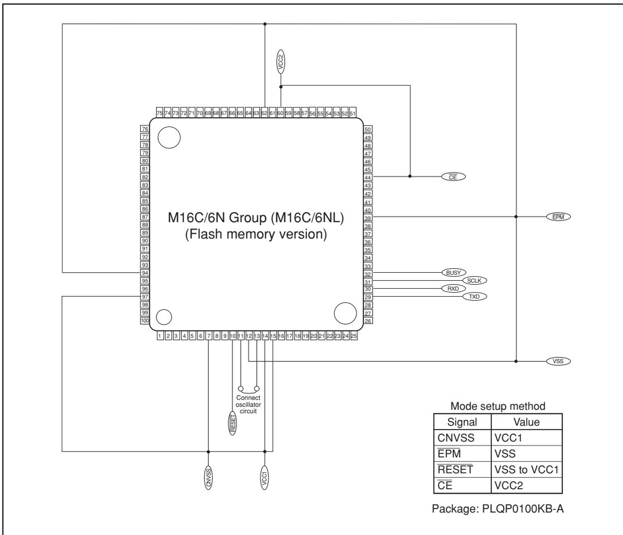
Figure 20.13 Pin Connections for Standard Serial I/O Mode (1)
