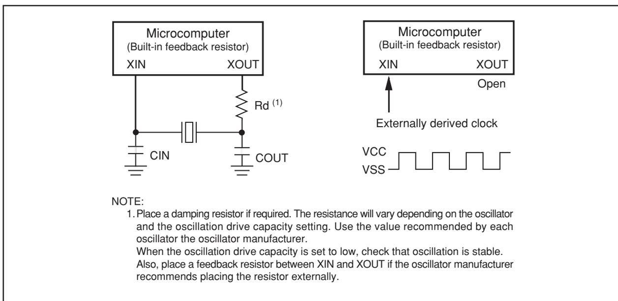
Figure 7.9 Examples of Main Clock Connection Circuit
