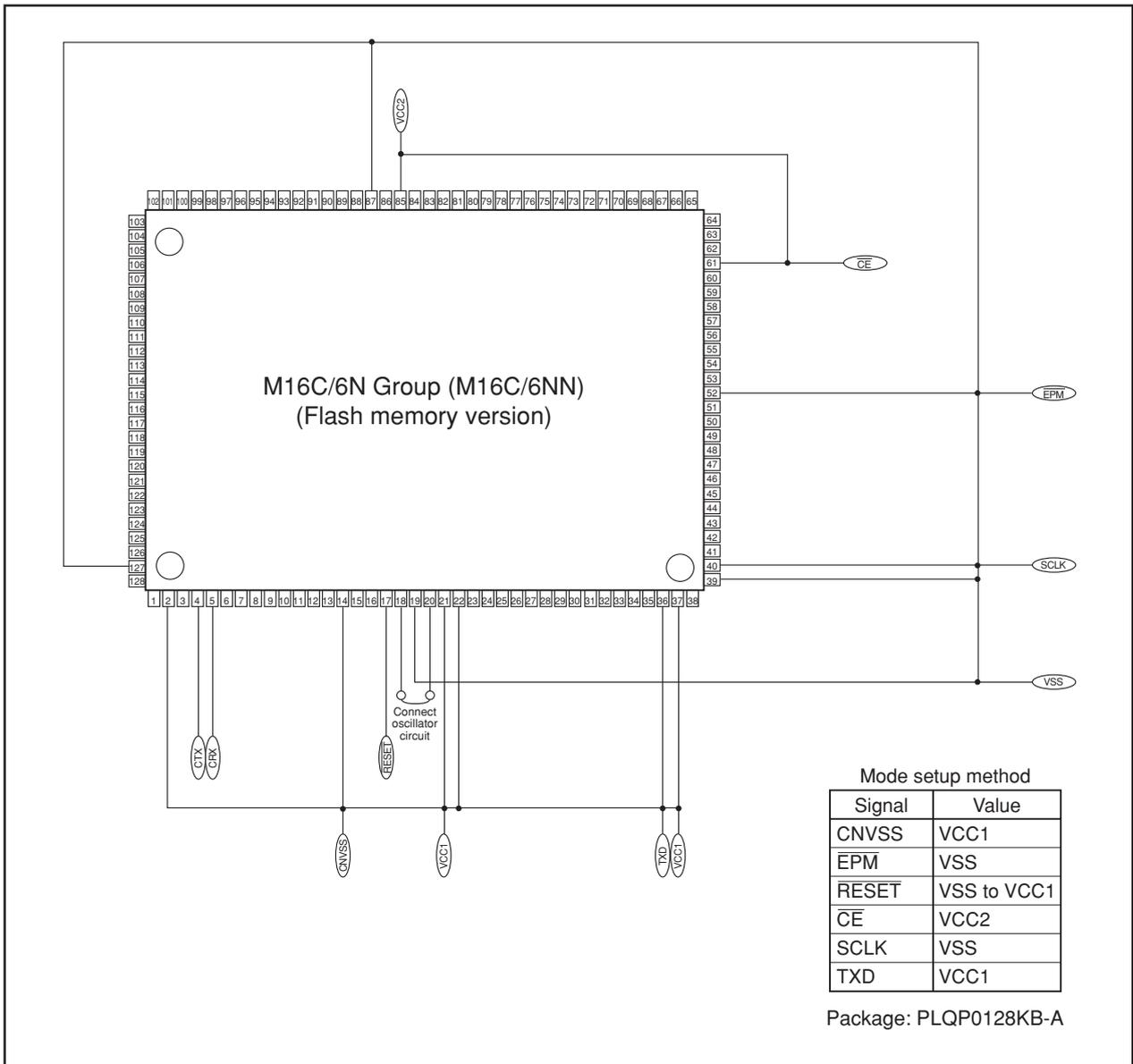
Figure 20.18 Pin Connections for CAN I/O Mode (2)
