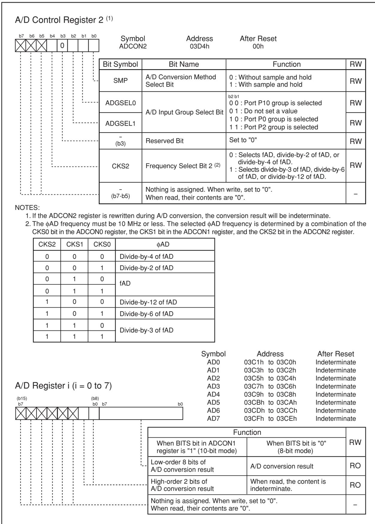
Figure 15.3 ADCON2 Register, and AD0 to AD7 Registers
