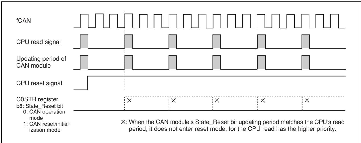
Figure 22.5 When Updating Period of CAN Module Matches Access Period from CPU
