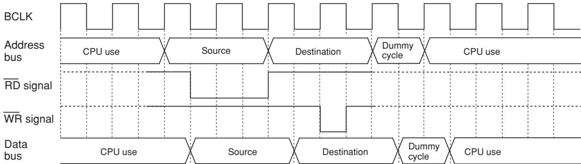
(4) When the source read cycle under condition (2) has one wait state inserted
