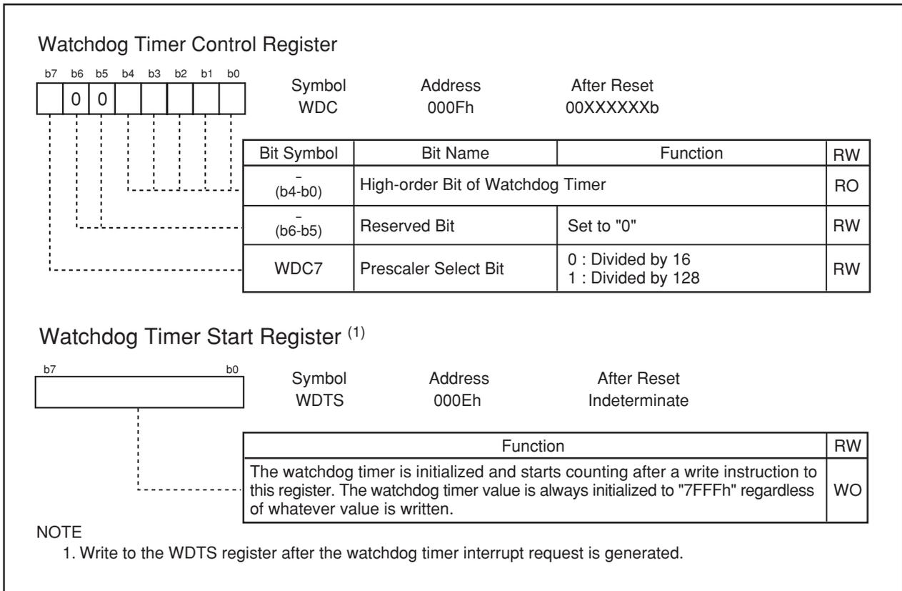
Figure 10.2 WDC Register and WDTS Register
