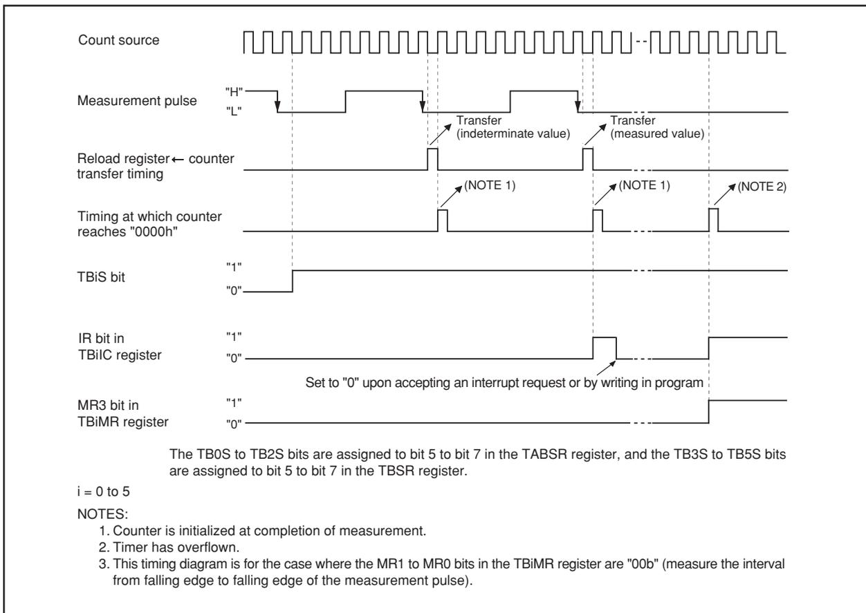
Figure 12.21 Operation Timing When Measuring Pulse Period
