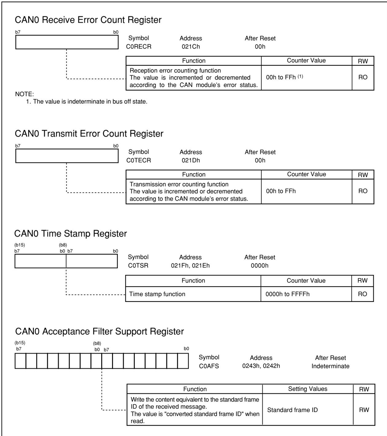
Figure 18.12 C0RECR Register, C0TECR Register, C0TSR Register and C0AFS Register
