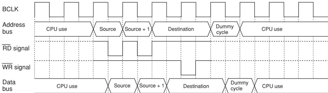
(3) When the source read cycle under condition (1) has one wait state inserted
