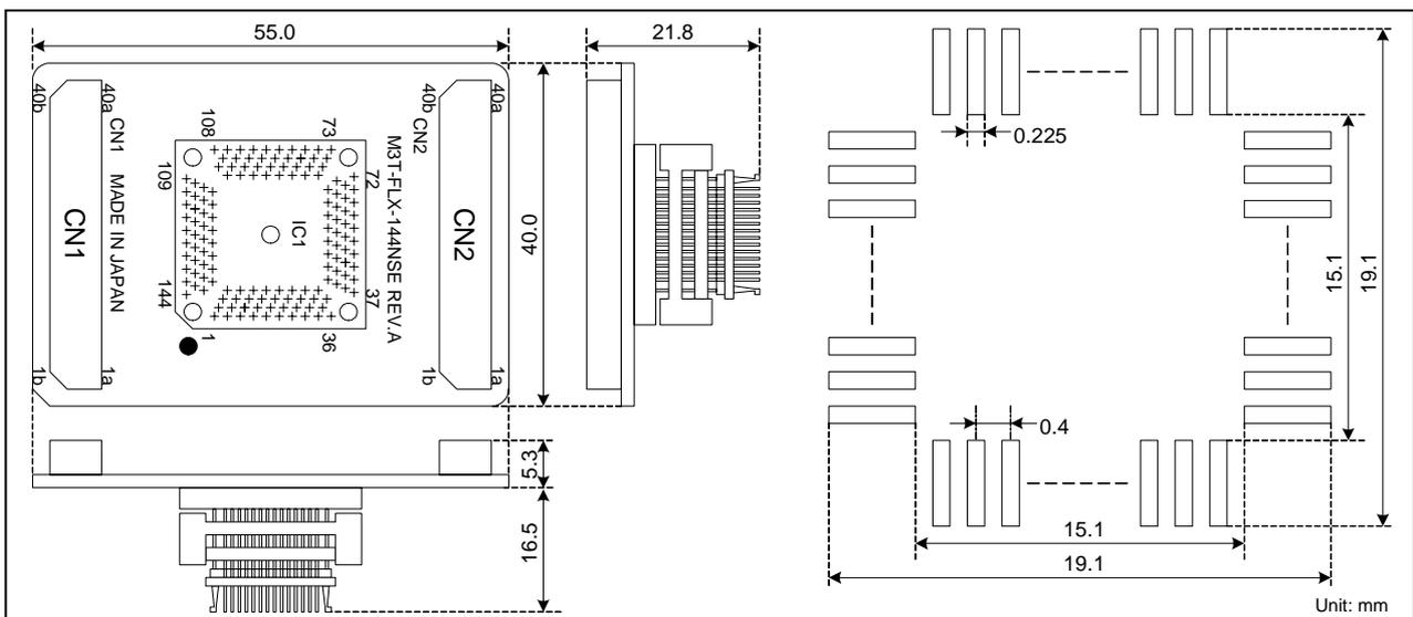
Figure 4 External dimensions and a sample foot pattern of the M3T-FLX-144NSE
