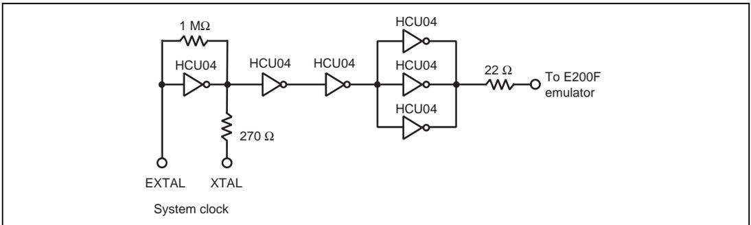
**Figure 12 Clock Oscillator**
