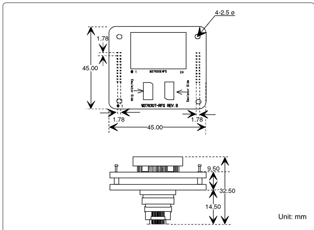
Figure 5.1 External dimensions of the M37630T-RFS
