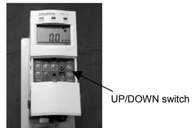
(7) Remove the calibration gas, check that the detected gas concentration is under that of the alarm value, and restore to the normal mode (by switching the maintenance switch to the center).
