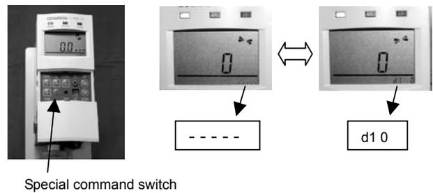
(4) Change the value by using the UP/DOWN switches (“△” or “▽”). When you are done, press the special command switch again, and the alternating display in the bottom right corner of the LCD display will become constant. The process is now finished.
