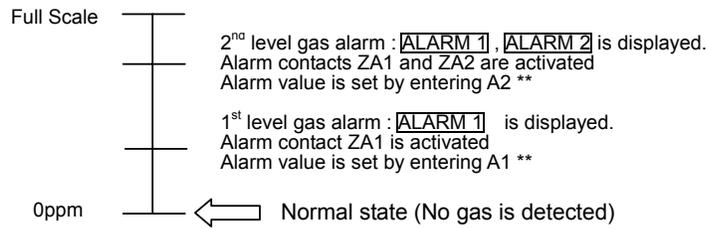
**L – L mode (1<sup>st</sup> level: Lower limit, 2<sup>nd</sup> level: Lower limit)**
