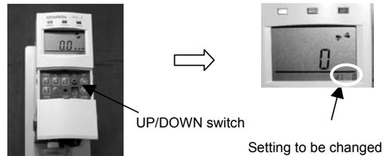
(3) Then press the special command switch, and the setting to be changed ( “LCD Screen Indication” in the table below ) and “—” will flash alternately.
