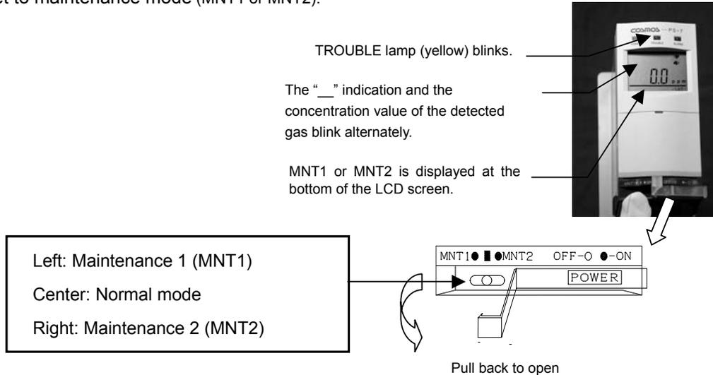
(2) Release the password lock. (Refer to 1-2 Releasing the Password Lock.)
