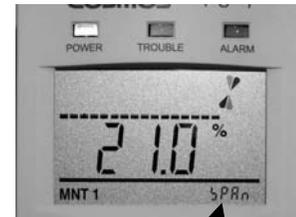
SPAN is displayed at bottom of the LCD screen
